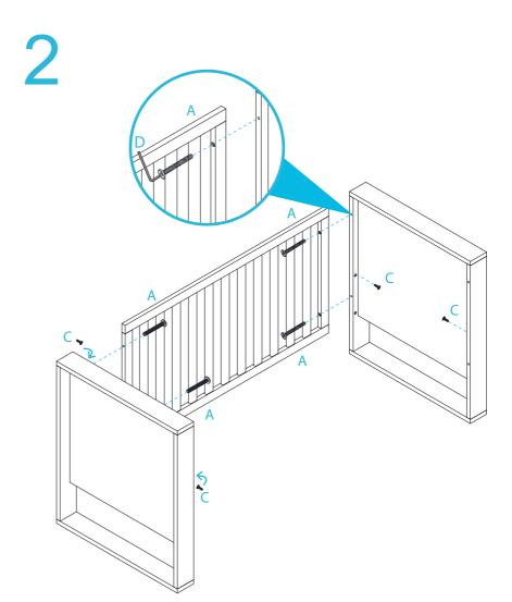
Find one of the side panels and attach to both end panels of the cot using 4x screws (A) in the holes as shown. Insert 4x screws (C) in the holes as shown. Tighten with the Allen key (D)
