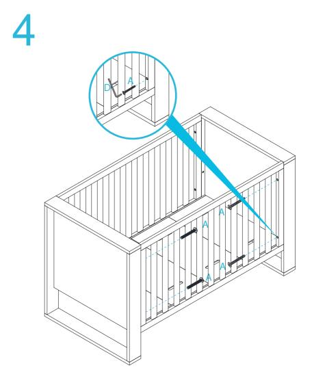
Slide the remaining side panel into place and attach using 4x screws (A) in the holes as shown. Tighten with the Allen key (D).
