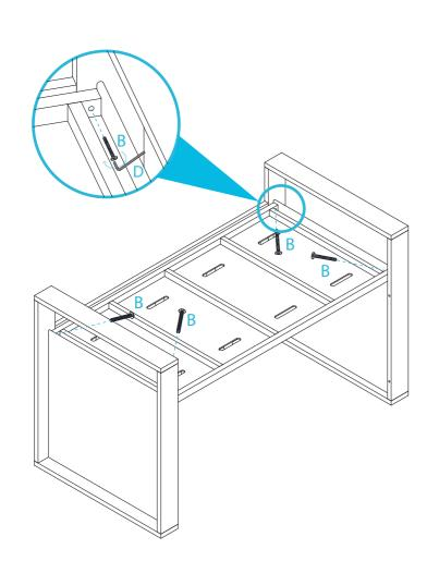
Attach the cot base at the required level using 4x screws (B) as shown, and tighten with the Allen key (D).
