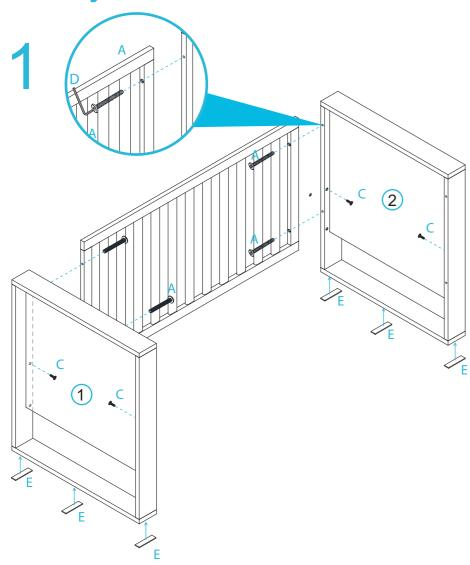
Find one of the side panels and attach to both end panels of the cot using 4x screws (A) in the holes as shown. Insert 4x screws (C) in the holes as shown. Tighten with the Allen key (D). Attach 6 x foot pads (E) to panels [1] and [2].
